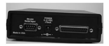
Figure 1a. P2RS Parallel to Serise Converter
